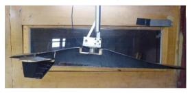
Figure 3. Experimental setup of 3x4 ft Michigan AFRL cruiser wind tunnel model.
