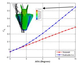
Figure 5. CFD and TRANAIR results of Hexafly  $C_L$  vs AoA showing strong leading edge vortices for the 15 degree AoA case.
