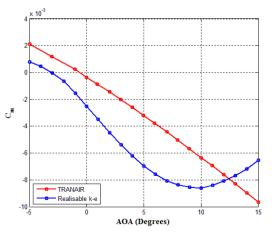
Figure 6. CFD and TRANAIR results of Hexafly  $C_m$  vs AoA.
