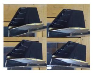
Figure 12. Tuft flow visualisation of the Michigan AFRL Cruiser vortex/fin interaction at (a) 0 degrees *AoA* (top left), (b) 5 degrees *AoA* (top right), (c) 10 degrees *AoA* (bottom left) and (d) 15 degrees *AoA* (bottom right).
