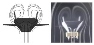
Figure 13. Comparison of vortex behaviour for Michigan AFRL cruiser seen in CFD (left) and smoke tunnel (right) at 15 degrees *AoA*.
