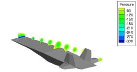
Figure 11. Vortex formation and fin interaction of Michigan AFRL cruiser (right) at 10 degrees *AoA*.
