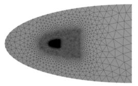
Figure 1. Half body mesh typical of the Michigan AFRL cruiser and Hexafly-Int vehicles containing approximately  $15 \mathrm{x} 10^6$  elements.
