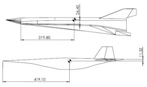
Figure 2. CoG location for Hexafly-Int (top) and AFRL Cruiser (bottom)
