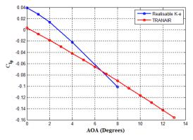
Figure 7. CFD and TRANAIR results of Hexafly roll moment coefficient gradient for increasing *AoA*.
