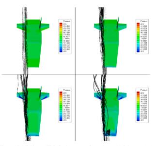
Figure 10. Michigan AFRL Cruiser vortex formation at (a) 0 degrees *AoA* (top left), (b) 5 degrees *AoA* (top right), (c) 10 degrees *AoA* (bottom left) and (d) 15 degrees *AoA* (bottom right).
